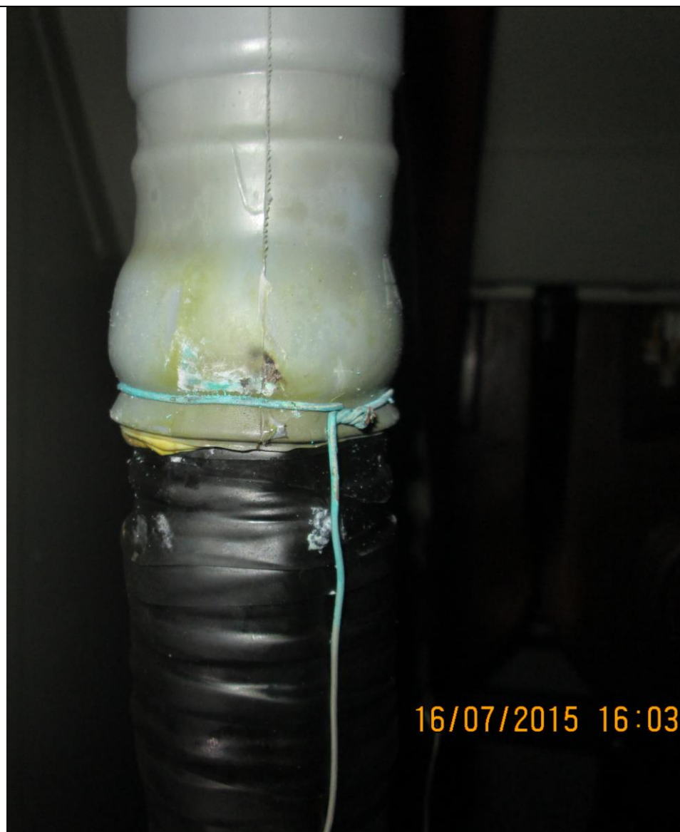
Visible Electrical treeing which originates from the point of touching with cable and the black insulation cover.
